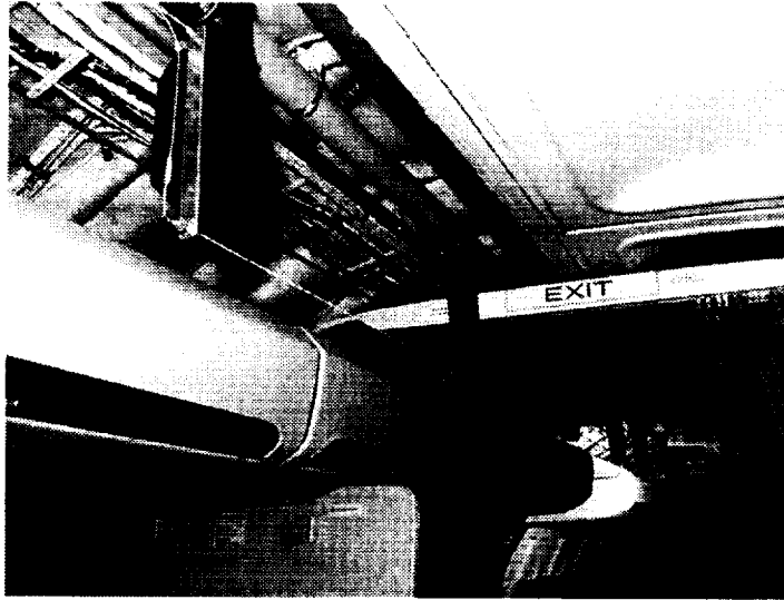
Figure 2.10. Cabin Long Wire (CLW) sensor. Both the wire and the small strip of metal, used in lieu of a ground plane, can be seen in this photograph.
